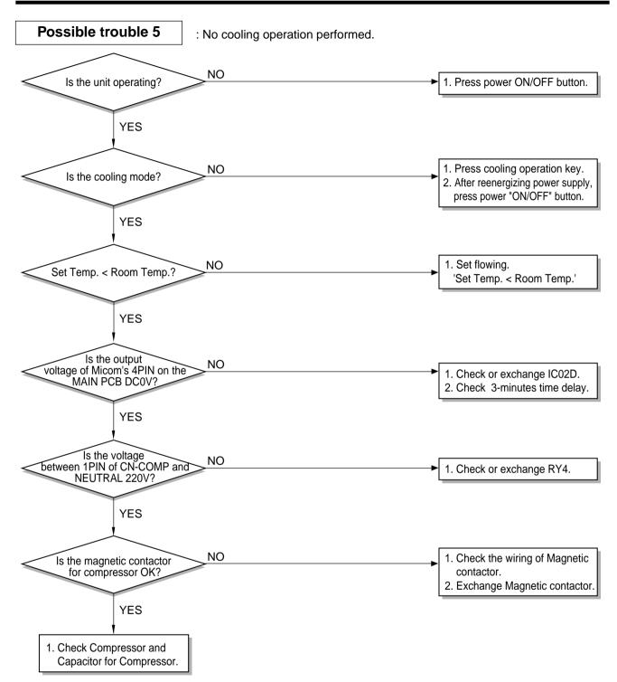
NOTE: 3ø model has not capacitor for compressor.
